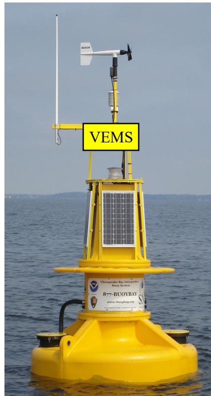
FIGURE 21: VEMS PLACEMENT ON SMART BUOY
