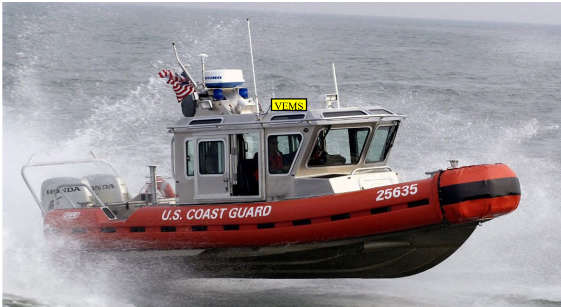
FIGURE 20: VEMS PLACEMENT ON PATROL BOAT
