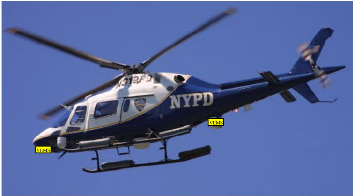
FIGURE 22: VEMS PLACEMENT ON HELICOPTER
